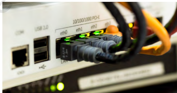
Figure 10.12: Cables connected to a network switch
