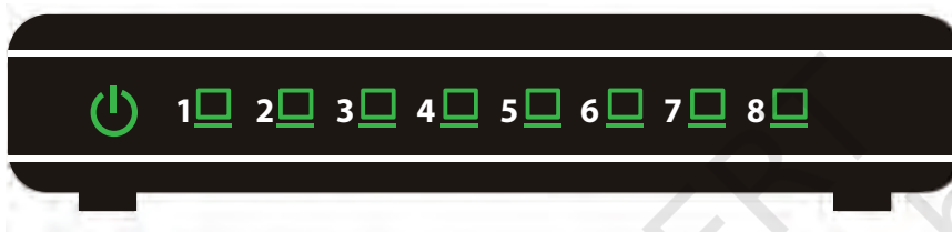
Figure 10.11: A network hub with 8 ports
