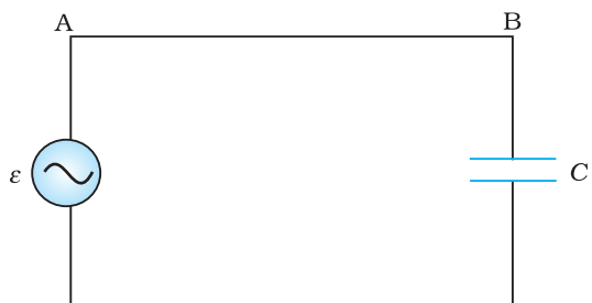
FIGURE 7.7 An ac source connected to a capacitor.
