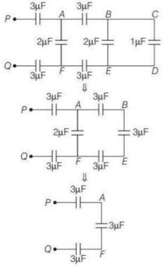
The equivalent capacitance between P and Q is given by  $\frac{1}{1} = \frac{1}{1} + \frac{1}{1} + \frac{1}{1} = 1\mu F$
