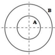
If  $D_1$  and  $D_2$  are the diameters of the inner and outer tubes, respectively, then the view factor  $F_{BB}$  is given by
