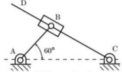
The magnitude of the relative sliding velocity of slider B with respect to rigid link CD is
