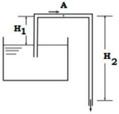
Assuming that the fluid is ideal and the reservoir is large, the velocity at point A in the siphon tube is:
